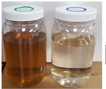
Fluid sample from chiller with UV-C with contaminant
