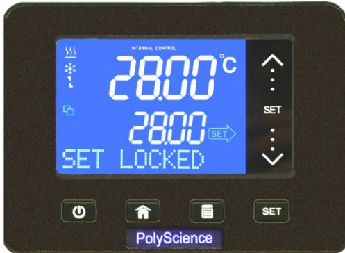
SET LOCKED – Read Commands Only Permitted
